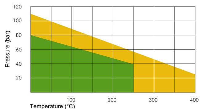
The P x T diagram above indicates the service limits for **NA-1002EU** considering the simultaneous influence of pressure and temperature (chemical suitability assumed). The green area represents the normal service limits, while the orange colored area shows the maximum application limits. For those cases, please consult our technical department.
