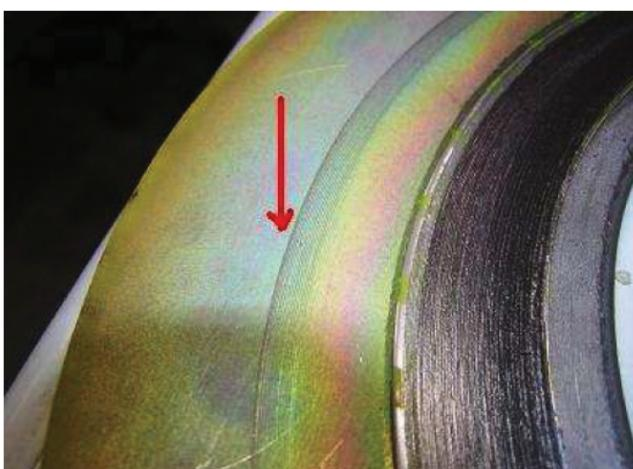
Figure 13: Flange raised face contact imprint on outer ring.
