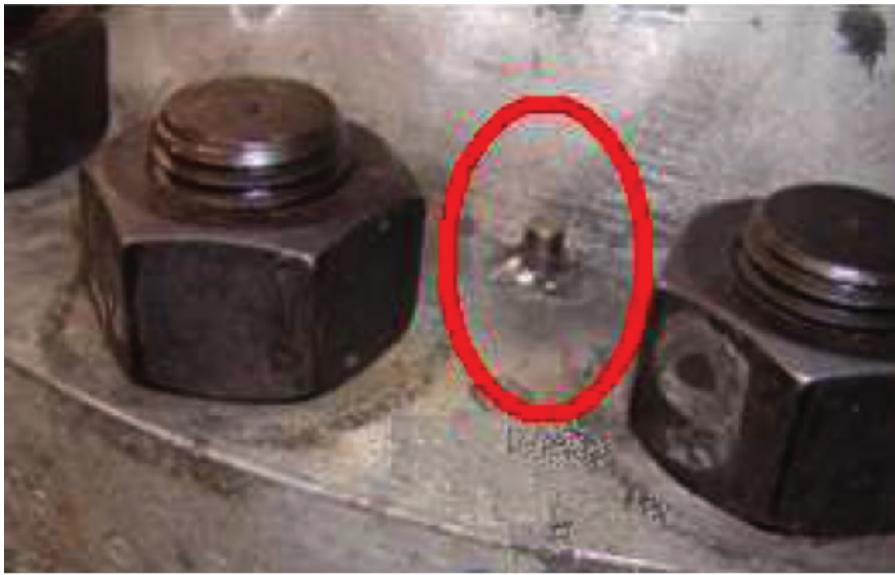
Figure 18: Measuring pin.
