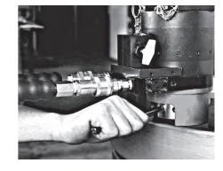
common for specific applications. Tensioning is especially effective on high-pressure flanges with large bolt diameters and critical joints, across industries such as oil and gas, wind, subsea, and power generation.
