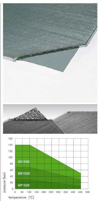
Because graphite sheets are fragile and therefor difficult to handle, we recommend the use of styles with metal insertions.
