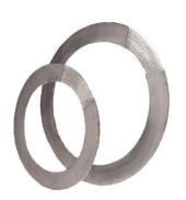
Corrugated metal gaskets with flexible graphite facings, style 905 Metalbest, have gained popularity in the marketplace in Class 150 and 300 ASME B16.5 flanges due to their ability to seal at low bolt loads.
