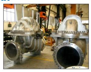
pressure to consider, the gasket needed would have to withstand the pump pressure of 435 psi (30 bar) without leaking. This customer contacted Teadit's engineering department for a sealing material recommendation for this application.
